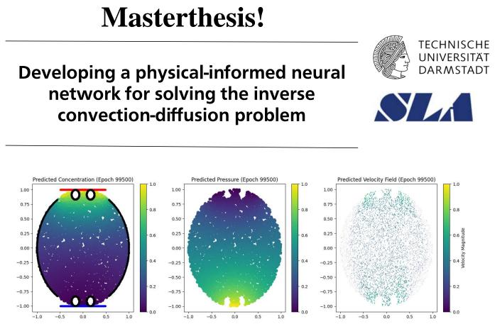
As part of the FlowForLife research project, a microfluidic supply network for 3D cell clusters is being developed. One aspect of the network design is the oxygen transport in the surrounding matrix. To characterize this, oxygen quenching luminescent particles are added to the surrounding matrix. The oxygen concentration can be determined at each particle.
